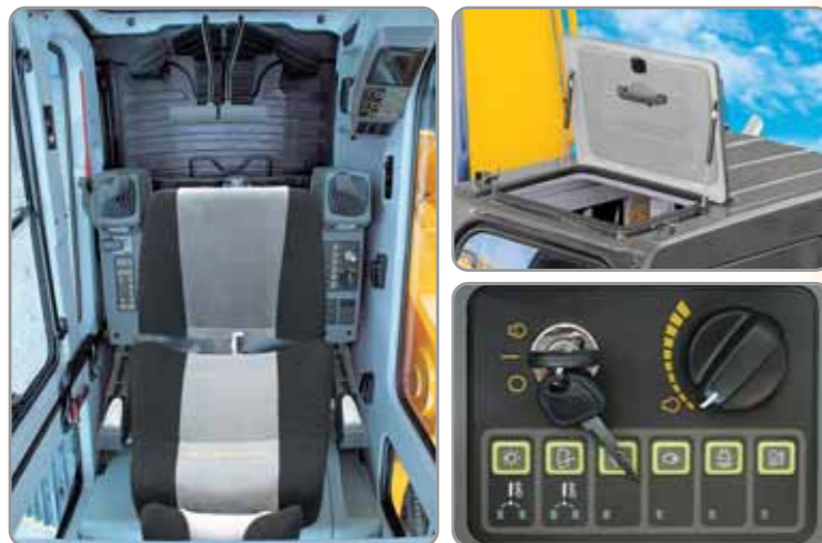
1 Wide, Comfortable Operating Space 2 Steel Cover Sunroof 3 Dial Type Engine Speed Switch and Key Switch
